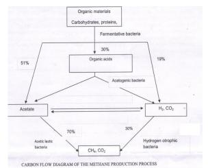
Figure 1. Flow chart of methane production
